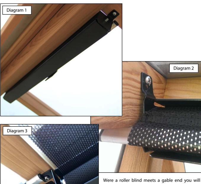
Were a roller blind meets a gable end you will need adjust the direction of the flange (diagram 2). Using an adjustable spanner clamp this onto the flange with the fixing hole in and bend it upwards. You will now be able to fix this inline with the other blinds.
